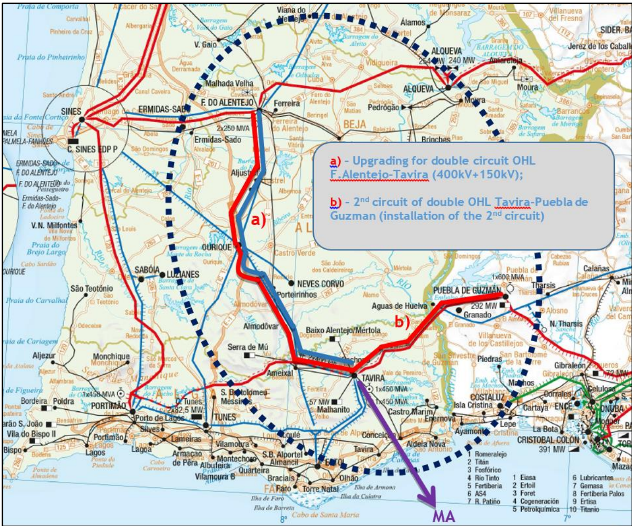
Figure 4 – Internal reinforcements in Portugal which were considered in order to accommodate the 1000MW flow between Portugal and Morocco (Med-TSO network studies)
