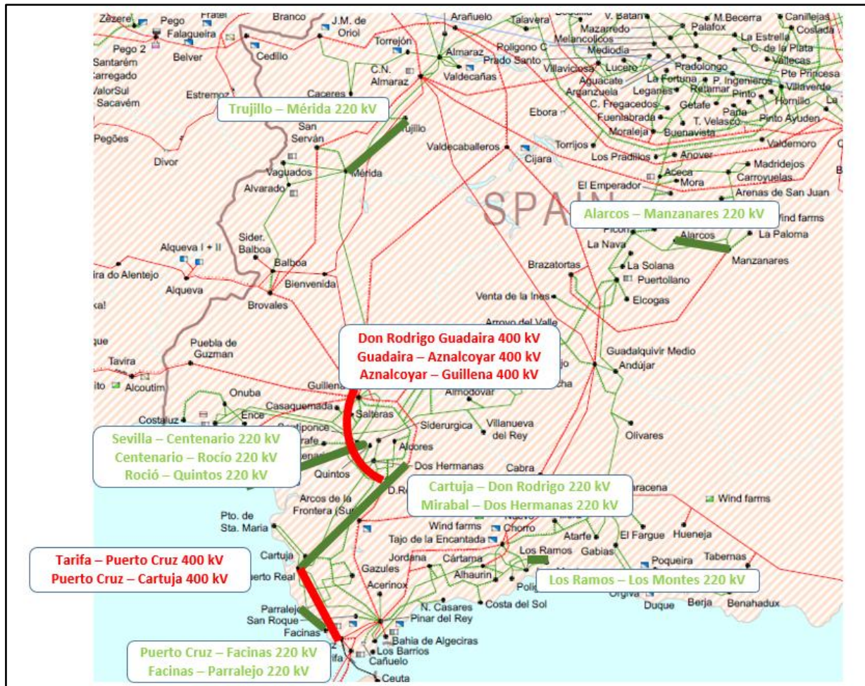
Figure 2 – Internal reinforcements in Spain which were considered in order to accommodate the 1000MW flow between Spain and Morocco (Med-TSO network studies)
