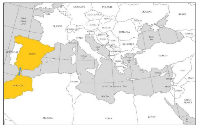
This project consists of a new interconnection between Morocco and Spain. In addition to the two existing links, the project consists of a third link, based on HVAC technology, which will increase the NTC between both countries by 600 MW or 650 MW (Morocco – Spain and Spain – Morocco respectively). The total length of the interconnection line is estimated at around 60km, corresponding to a 30km subsea cable and a 30km overhead line.
